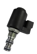
3/2 Direct acting spool type Max. pressure: 210 bar (3000 psi) Max. flow: 10 lpm (2.6 gpm)
