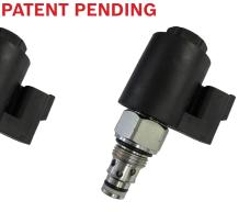
2/2 Pilot operated poppet type Normally open Max. pressure: 350 bar (5000 psi) Max. flow: 40 lpm (11 gpm)
