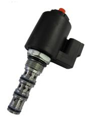
4/2 Direct acting spool type Max. pressure: 210 bar (3000 psi) Max. flow: 10 lpm (2.6 gpm)
